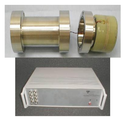
The picture above-left shows the Transmitter's electronics modular design for the 8 strain measurements; on the upper right, the electronics are shown in a rapid-prototype housing prior to insertion in a metal coupling. The exterior of the coupling, with a glass laminate induction power pickup coil assembly is shown in the lower left picture. The Receiver (digital to analog outputs device) is shown on the lower right.
